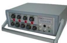
Model S-50: Measures up to 50 electrodes of two to four independent CMAS probes; also measures corrosion potentials, temperature and other parameters simultaneously from four independent CMAS probes, three pH or three ORP probes, or three other transducers for parameters such as conductivity, humidity, flow, and pressure.
