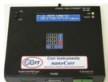
Model F-II-10(New): Measures one probe with up to 10 electrodes. It has the following features: • 0.005-50mm/yr range • 15seconds response time • On-board data storage • USB port for data storage or data transferring • 120/220VAC or 9-30V DC Power • 4-20mA/RS-232/RS-485 outputs • 7.2"x5.3"x2.25" size
